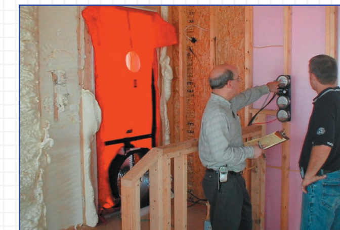
A blower door test was conducted to measure airflow, which proved that the most significant reduction in airflow was the result of the Icynene® application alone.
